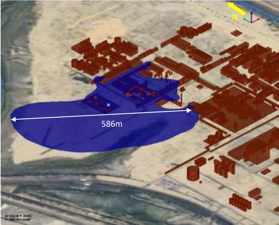
Figure 84: 3D view of ERPG3 @ 20000 ppm
