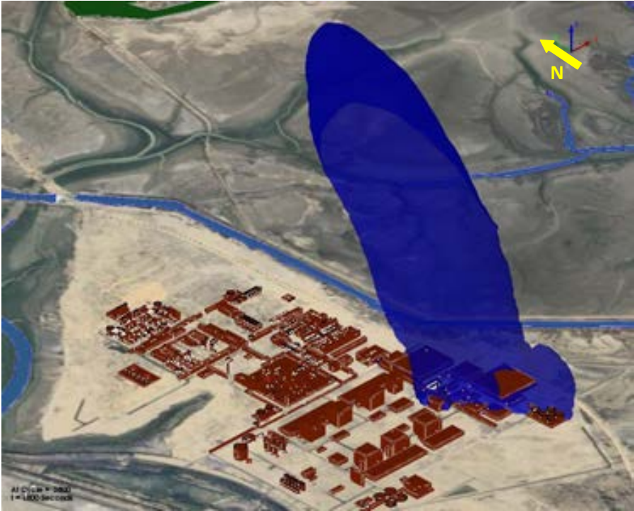
Figure 34: 3D plot view of IDLH @ 10 ppm
