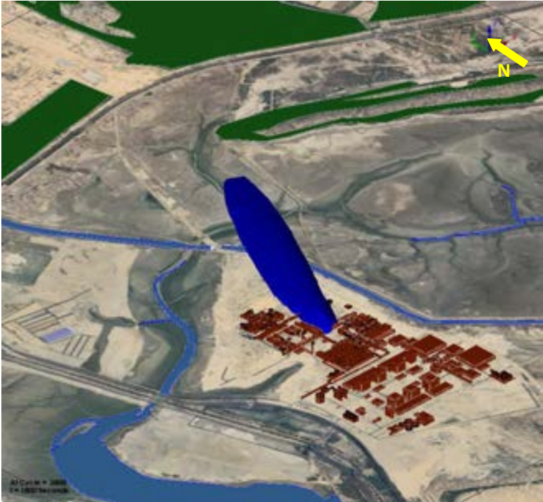
Figure 25: 3D plot view of IDLH @ 50 ppm
