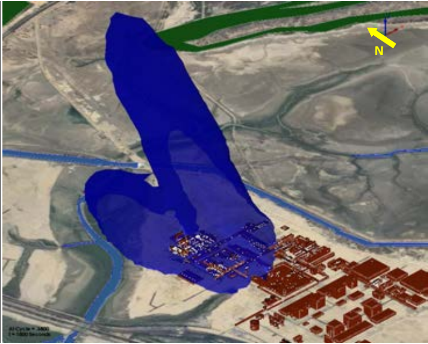
Figure 60: 3D plot view of IDLH @ 50 ppm
