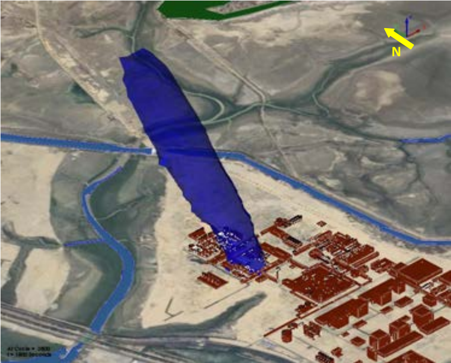
Figure 63: 3D plot view of IDLH @ 50 ppm
