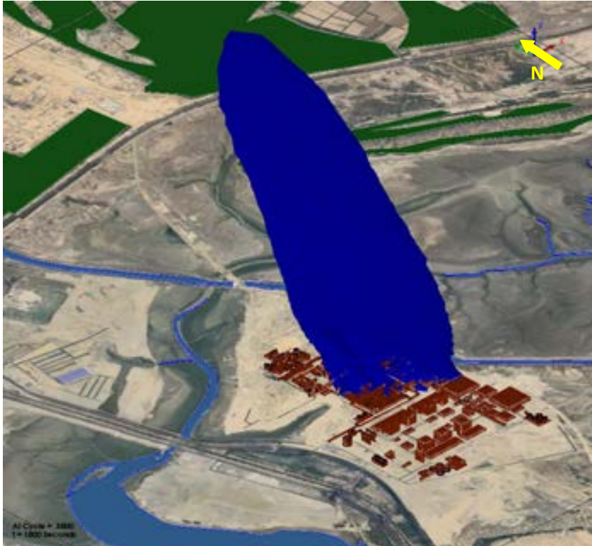
Figure 28: 3D plot view of IDLH @ 10 ppm
