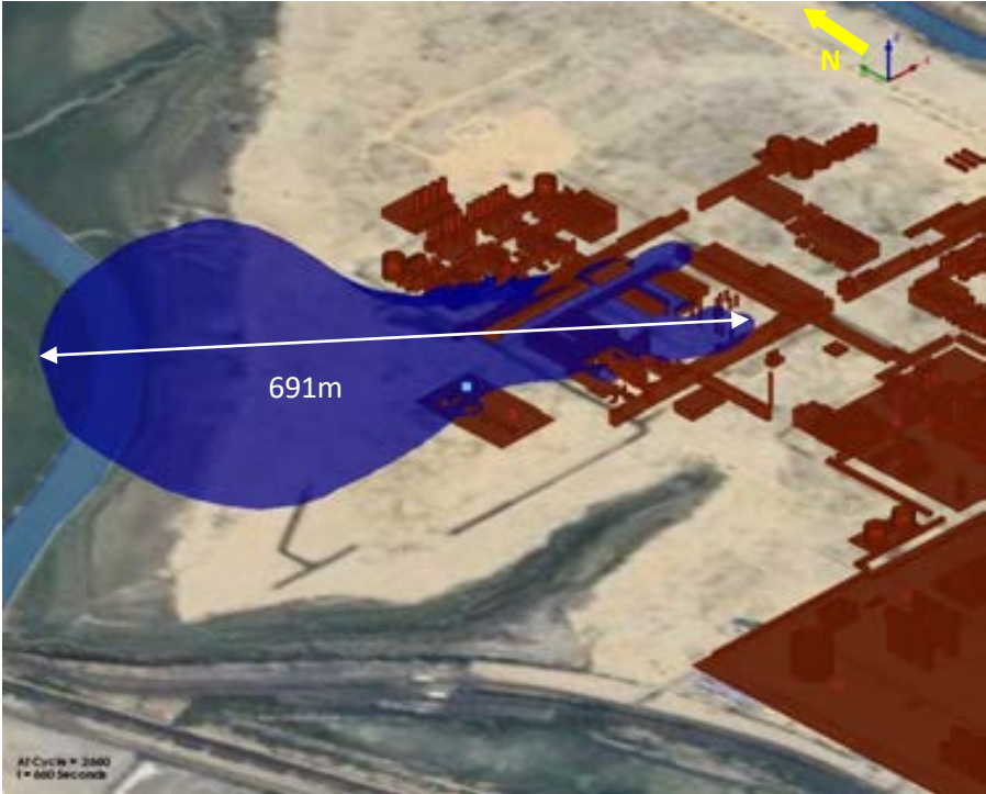
Figure 75: 3D view of ERPG3 @ 20000 ppm
