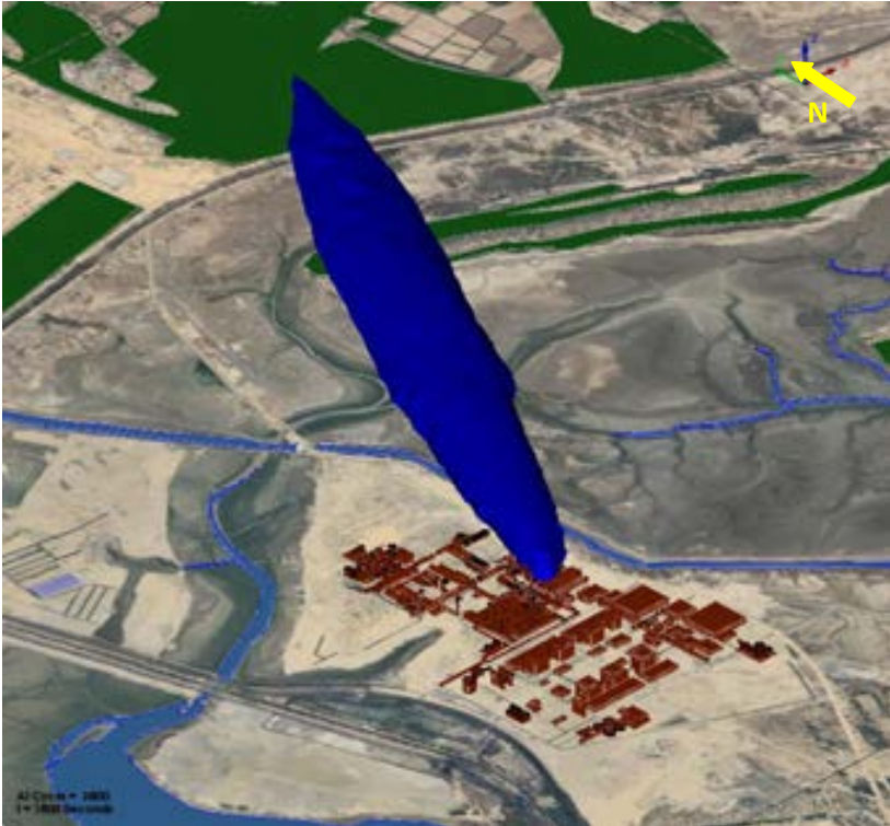
Figure 31: 3D plot view of IDLH @ 10 ppm
