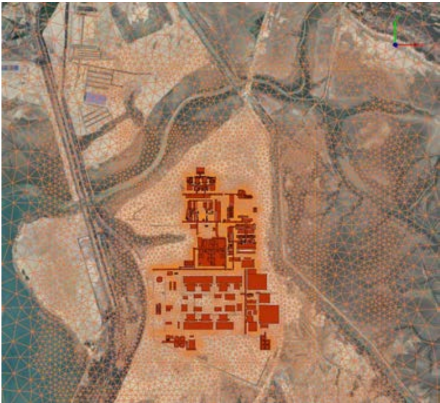
Figure 11: 2D Mesh considered for dispersion simulations
