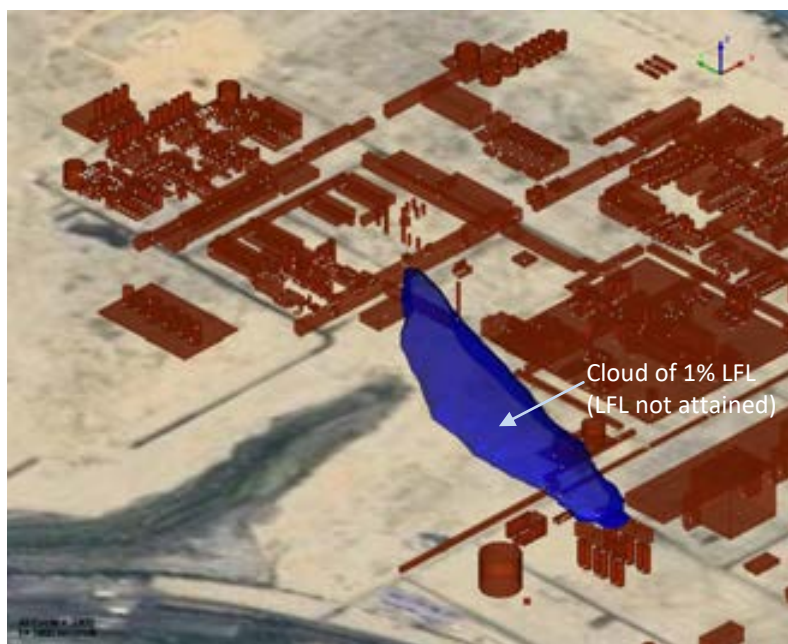
Figure 97: 1% LFL Cloud extent of Methane (100mm)
