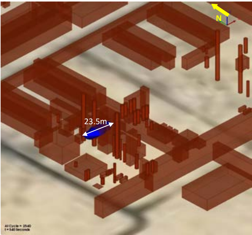
Figure 40: 3D view of ERPG3 @ 20000 ppm
