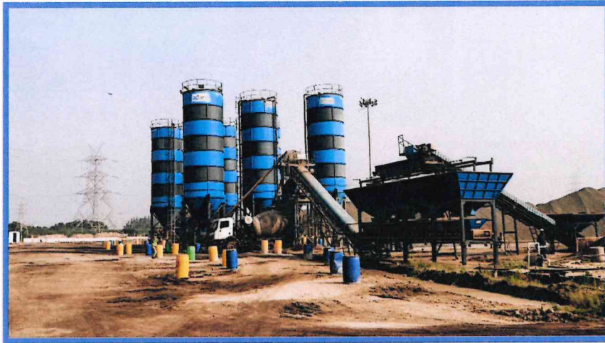
Batching Units / Facilities have been set up inside the premises to avoid fugitive emission due to long distance transportation.
