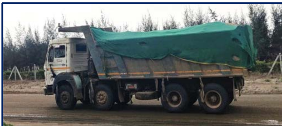
Material Covered with Sheet during transportation
