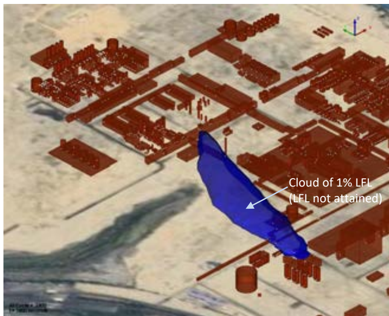
Figure 97: 1% LFL Cloud extent of Methane (100mm)
